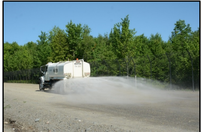
Water truck used for dust suppression
